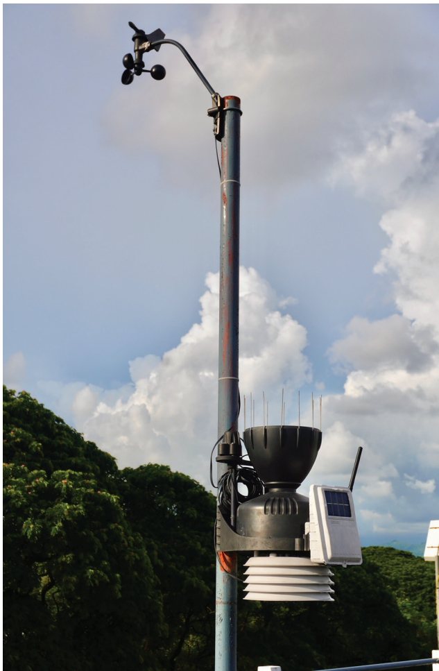
Figure 6. Davis Automated Weather Station
