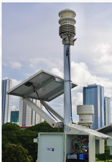
Figure 2. Lufft AWS at the Manila Observatory with the upgraded renewable power system.
